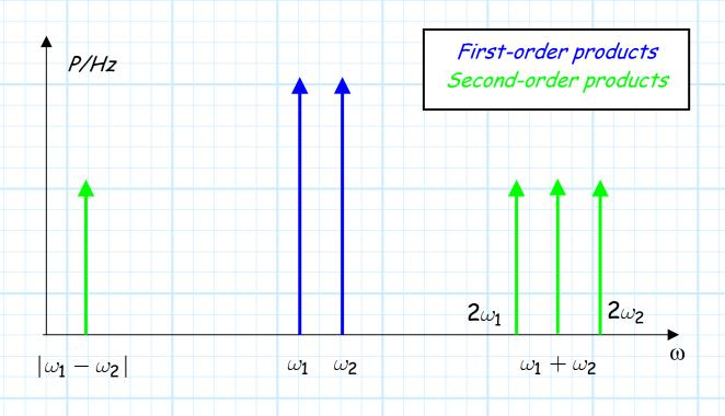
Note that the new terms have a frequency that is either much higher than both  $\omega_1$  and  $\omega_2$  (i.e.,  $(\omega_1 + \omega_2)$ ), or much lower than both  $\omega_1$  and  $\omega_2$  (i.e.,  $|\omega_1 - \omega_2|$ ).
